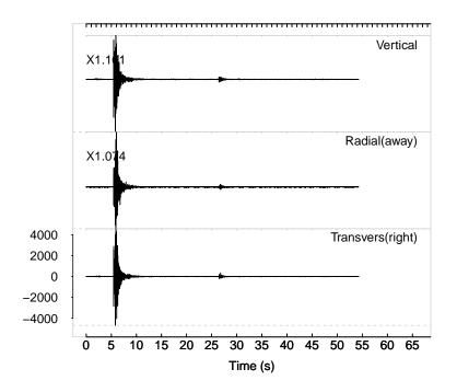
Next we extract information from the seismic structure that tells us when the P and S-arrival were estimated. This information is stored in the pickfile structure, but we want to know how many seconds paste the start of the trace the arrivals came in, so we can window that portion of the trace for hodogram analysis.
